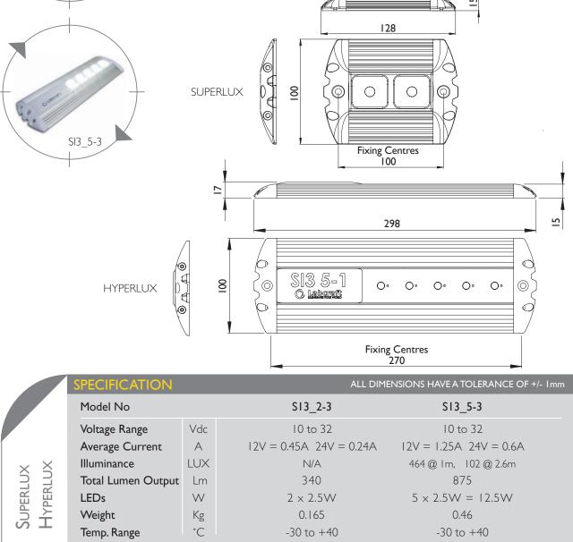
\*LED life is directly related to the running temperature within the LED. This product has been designed using the LED manufacturer's data to achieve 50,000 hours assuming an ambient temperature of 25°C. At this point light output may have decreased by 20%
