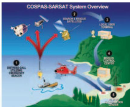
The GPS enabled EPIRBs and PLBs have built-in transmitters that will typically alert the rescue services within 3 minutes. These models are capable of providing positional accuracy of +/- 62 Metres and position updates every 20 minutes, given a clear view skyward.
