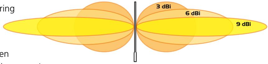
the gain, the omnidirectional pattern is squashed in a vertical plane and is enhanced in a horizontal plane. This expands the signal's coverage. A high gain antenna will therefore give increased coverage on flat terrain but the elevation will be limited making it unsuitable in mountainous regions.
