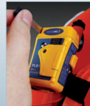
easy deploy retractable antenna
