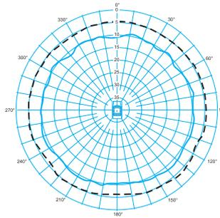
This pattern shows that the Phasemaster™ antenna is meeting the gain and omnidirectional performance we have stated in our specifications. The antenna is producing a "textbook" pattern and is delivering 4.5dB gain. This antenna is an excellent performer and is highly recommended for any roof mount application.
