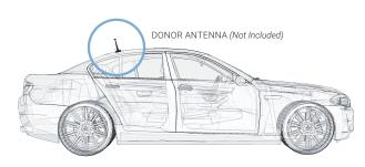
Mount your **Donor Antenna** on the exterior of the vehicle, towards the rear, according to its design, and the type of vehicle it's being used with. Make sure you consider the cable connection to the Cel-Fi GO unit with your location choice.
